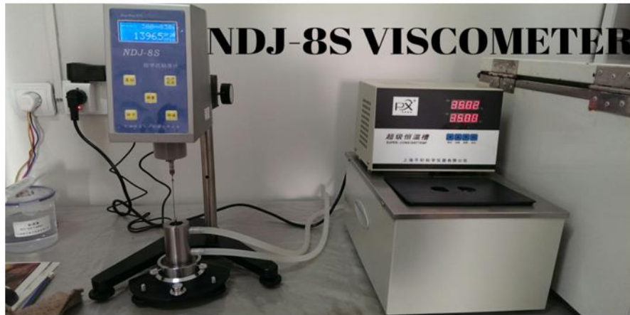
Fig. 1. NDC-8S brand viscometer (measurement limit of the device is up to 2 \cdot 10^6 mPa·s).
