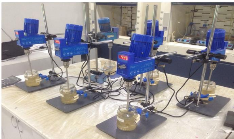
Fig. 3. Preparation of hydrogels of cross-linked hydrophilic polymers
